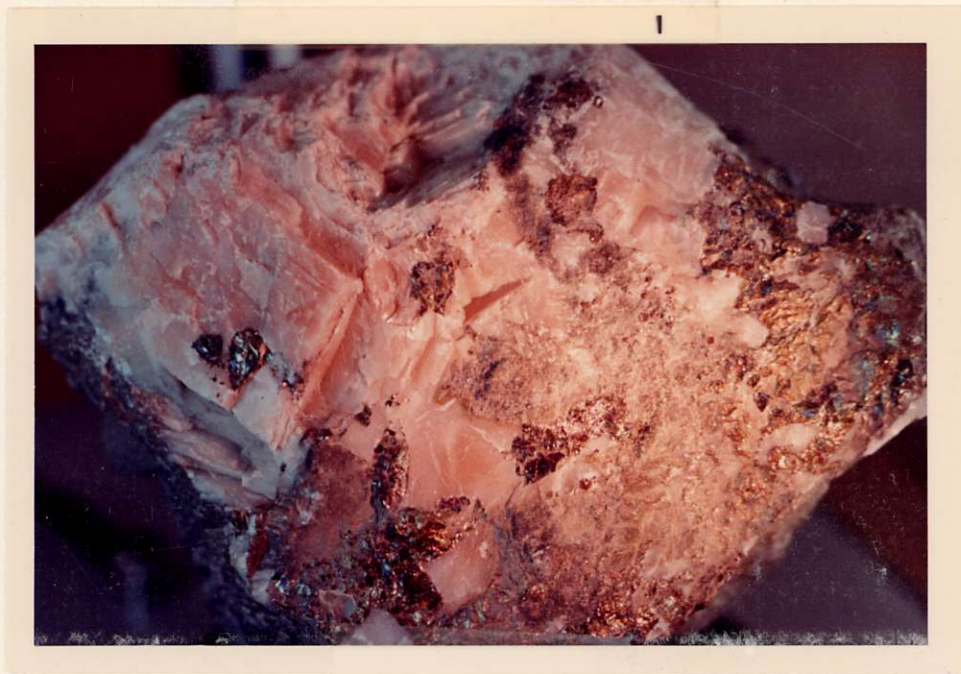
Figure 12. Secondary Calcite With Disseminated Chalcopyrite.
