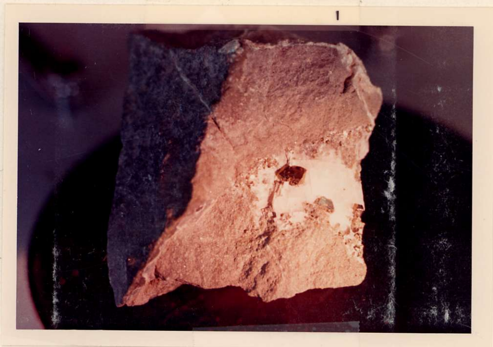
Figure 30. Calcite And Crystalline Pyrite In Epidote Skarn.
