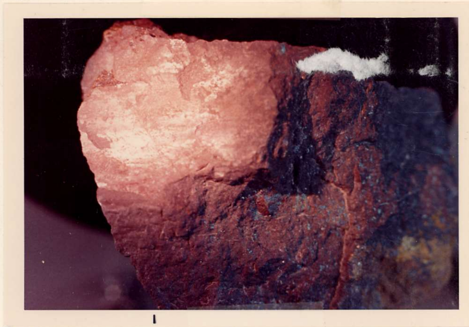
Figure 22. Post-ore Slickenside in Magnetite.
