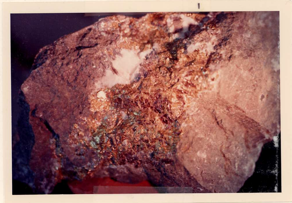
Figure 29. Calcite And Massive Chalcopyrite In Epidote Skarn.
