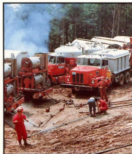
Fracing the Kubacki #1 well in Grandview Township, Ohio.
