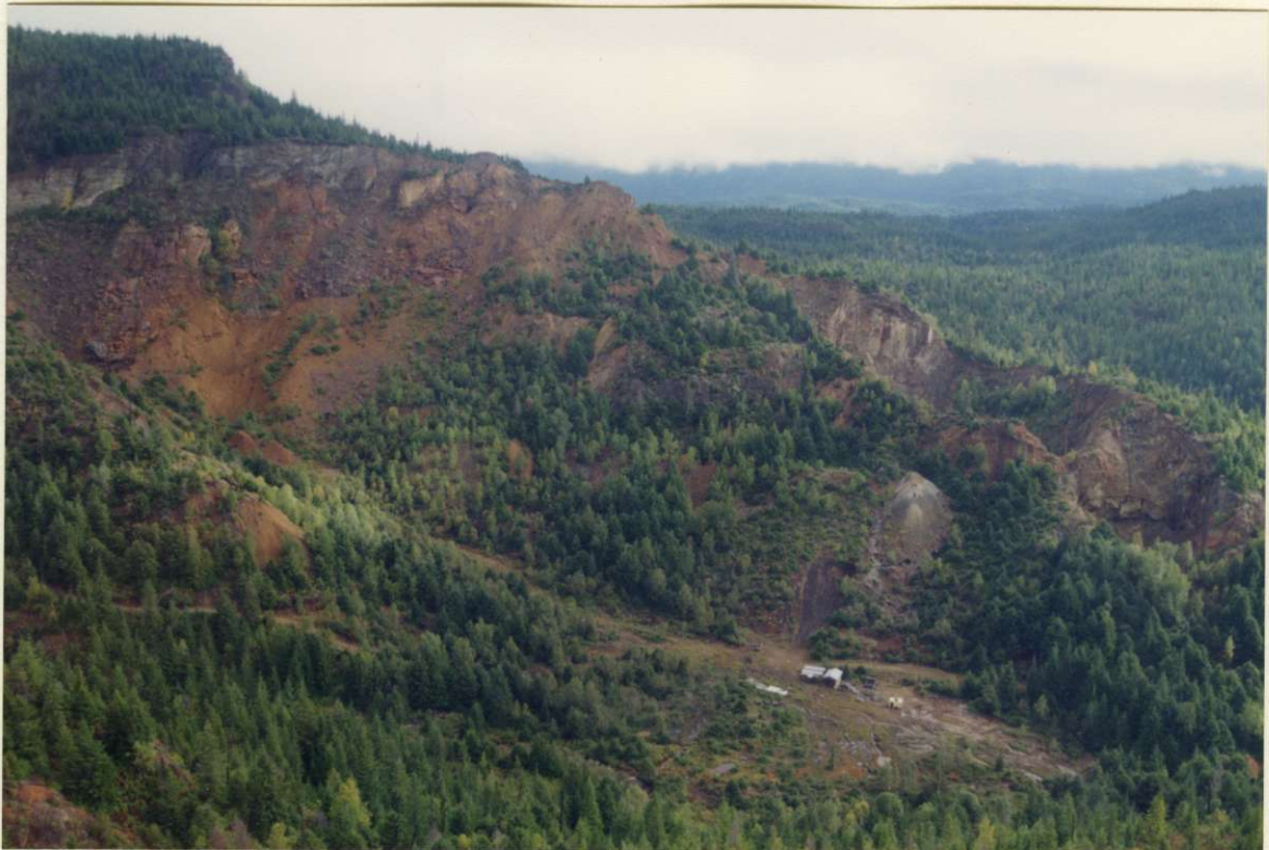
AERIAL VIEW OF HIDDEN CREEK OREBODY WHICH PRODUCED 21,681,000 TONNES OF 1.6% Cu, 0.17 g/t Au, 9.25 g/t Ag AND BOASTS RESERVES OF 13,600,000 TONNES OF 0.75% Cu.
