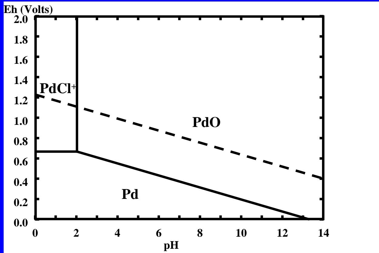
Eh – pH Diagram for the Pd-Cl system at 25 °C.
