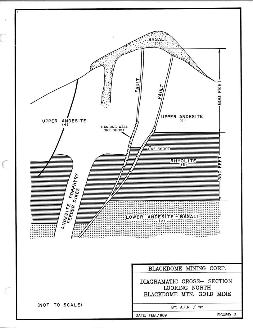
on the Blackdome property. All of the veins are more or less gold and silver bearing; however, mineable high grade ore-bodies are restricted principally to the South Mine segment of the No. 1 vein which is 4000 feet long from Section 12+750 N to Section 11+550 and is extensively developed by underground workings.
