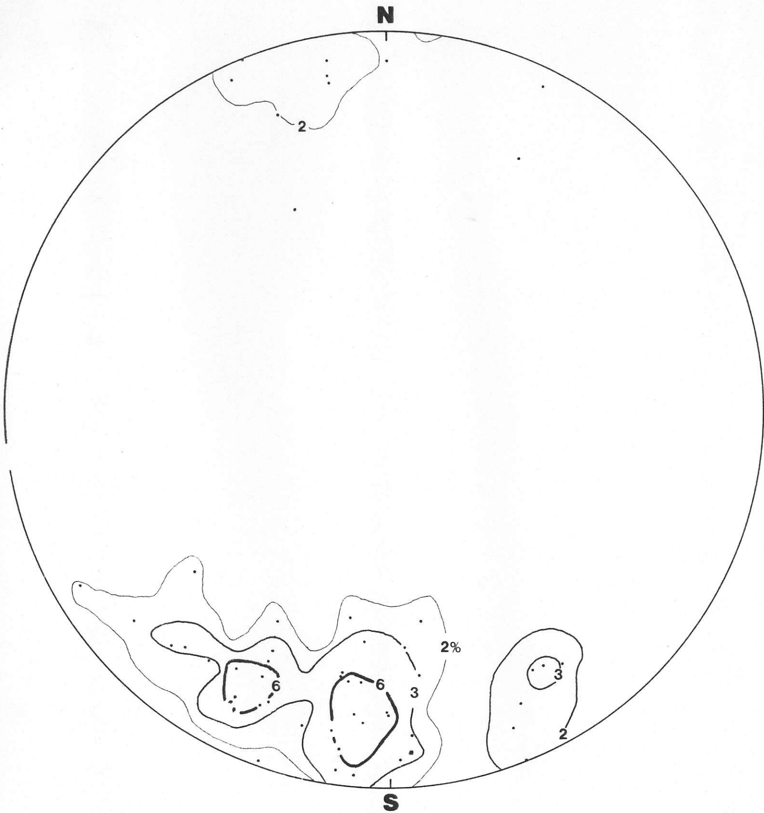
FIG 2 pole diagram of 53 "ac" joints
