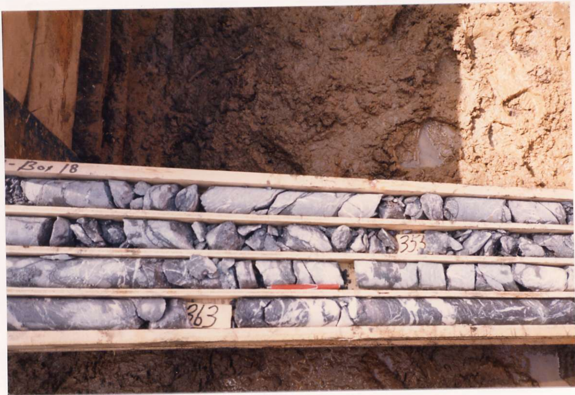
86-Roll 2-16 Core from T-86-51 showing multiple quartz veins cutting a purple andesite breccia.
