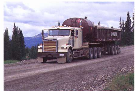
Specially designed trucks haul concentrate from the Kemess South mine to the rail-head at Mackenzie and backhaul fuel and grinding steel to the mine site.
