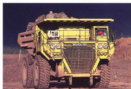
The primary haulage equipment at Kemess is the Canadian-made Euclid R260 truck. Tire life on each of the 13 trucks in the fleet has been doubled since Northgate acquired the mine.
