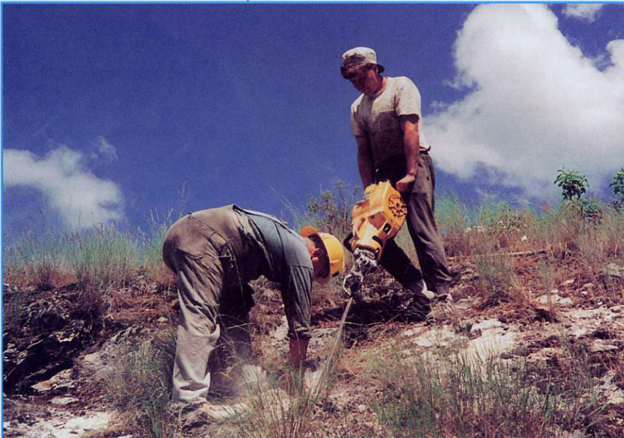
Left: Trenching the Summit gold discovery. Initial trenching revealed a 30 foot wide zone, averaging 0.287 oz/t gold.
