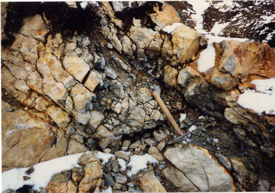
Figure 5. Altered breccia with sericitic tuff fragments and siliceous matrix/veinlets. The yellowish stain is reportedly jarosite, a common constituent of limonitic gossans. (R#45-12a)
