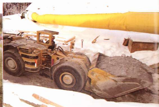
An underground scoop brings a load of mineralized material up the ramp to surface for stockpiling.
