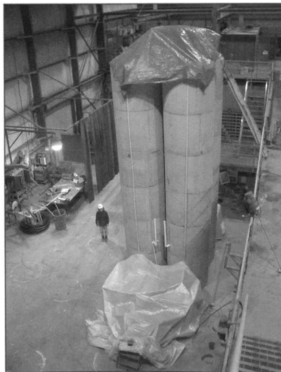
Test columns for oxide copper leaching
