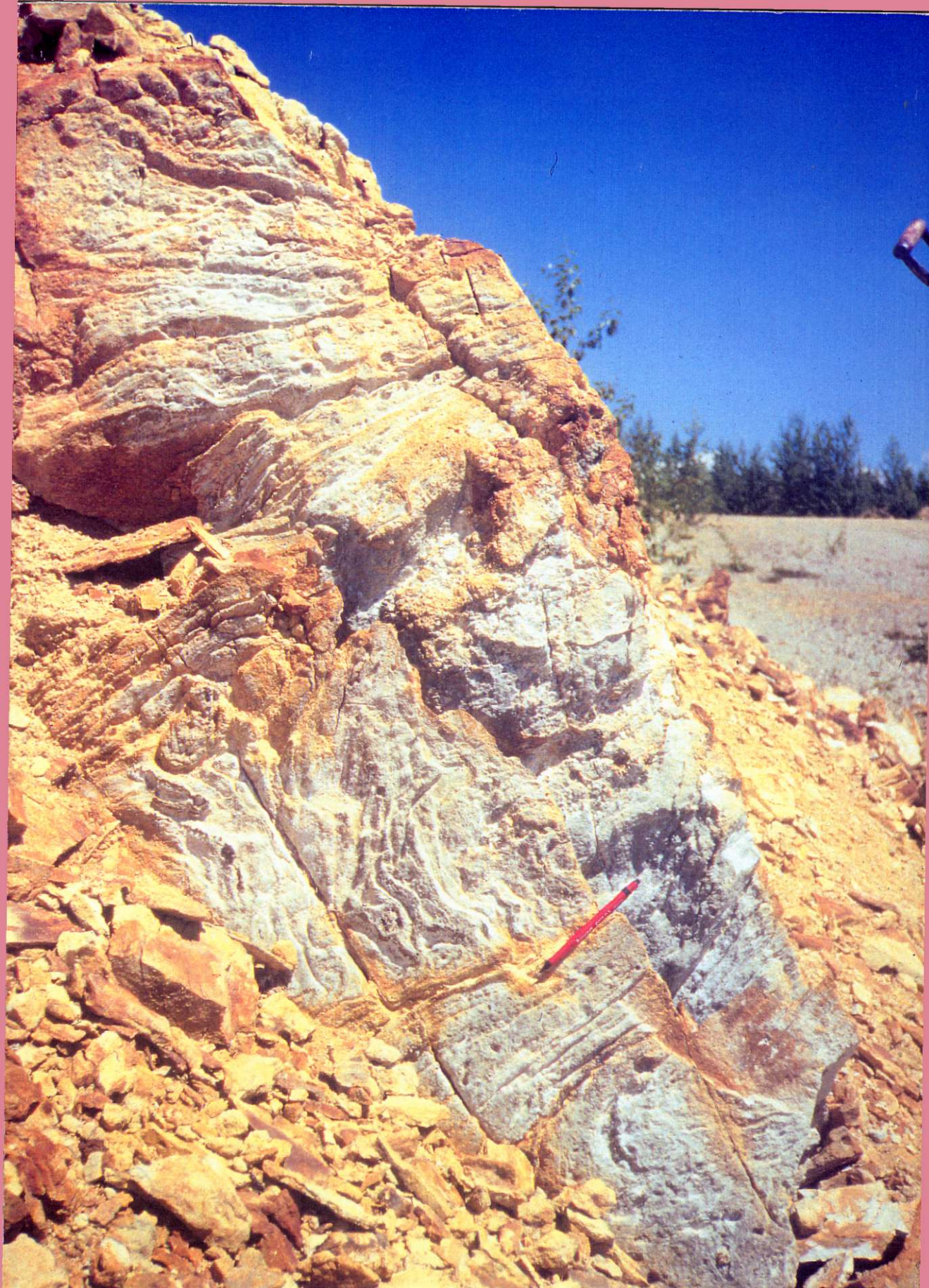
Strongly oxidized, quartz-sericite-pyrite altered, flow-banded rhyolite exposed on the north side of the Granisle pit along the uppermost bench. Similar rhyolitic intrusions occur elsewhere on the Newman Peninsula and are believed to be part of the Eocene Babine intrusive suite (Ebr)
