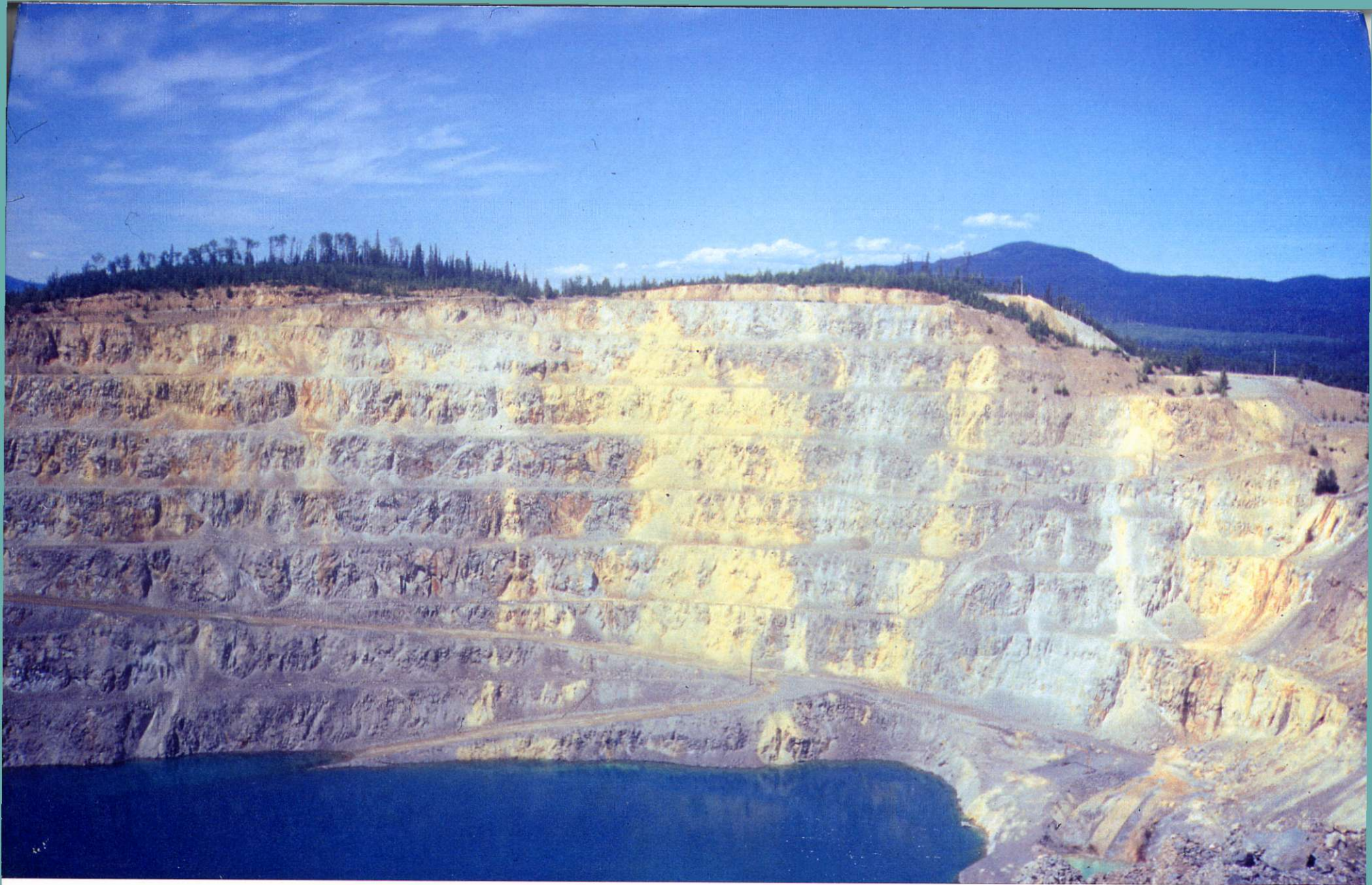
View looking north across the Granisle open pit. The Granisle mine produced 214 300 tonnes copper, 6 833 kg of gold and 69 753 kg silver from 52.7 million tonnes of ore between 1966 and 1982. Copper occurs within and peripheral to biotite-feldspar and quartz-biotite-feldspar porphyry intrusions of Eocene age (EBp).
