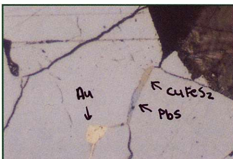
Several gold grains up to 10 \mu\text{m} , occur along fractures with chalcopyrite (dark yellow) and galena (silver-grey).
