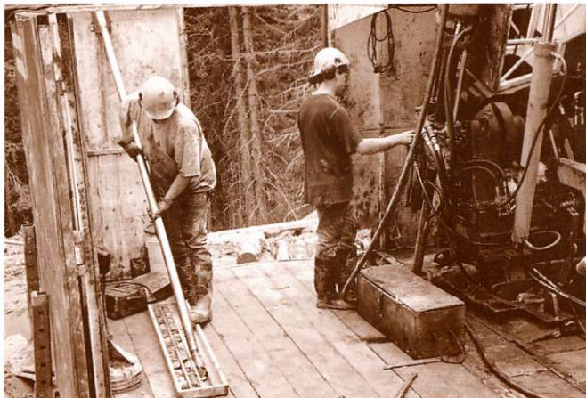
Kevin Cright extracts drill core from hole BC01-08 at the Bonanza Ledge. Gene Harris, at right, is operating the diamond drill. This hole returned 0.452 oz. gold/ton over 15.0 feet in the B.C. Vein extending its strike length to 3,300 feet.
