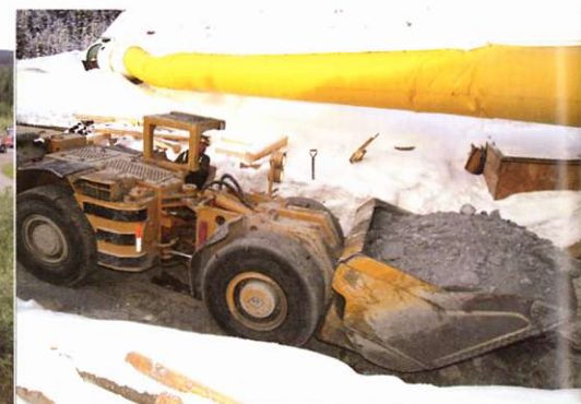
An underground scoop brings a load of mineralized material up the ramp to surface for stockpiling.
