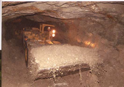
Hauling mineralized material with an underground scoop from the Bonanza Ledge Zone.
