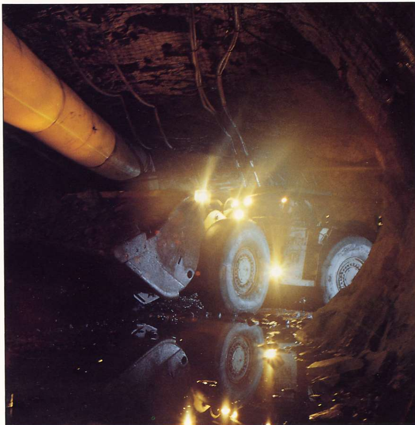
L.H.D. unit delivering ore to draw point, Williams gold mine, Hemlo, Ontario.
