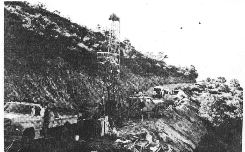
Recent diamond drilling on Gamin's Golconda project in northwestern Arizona tested two of nine known mineralized veins and revealed that the gold/silver/zinc/copper/lead mineralization extends to considerable depths.
