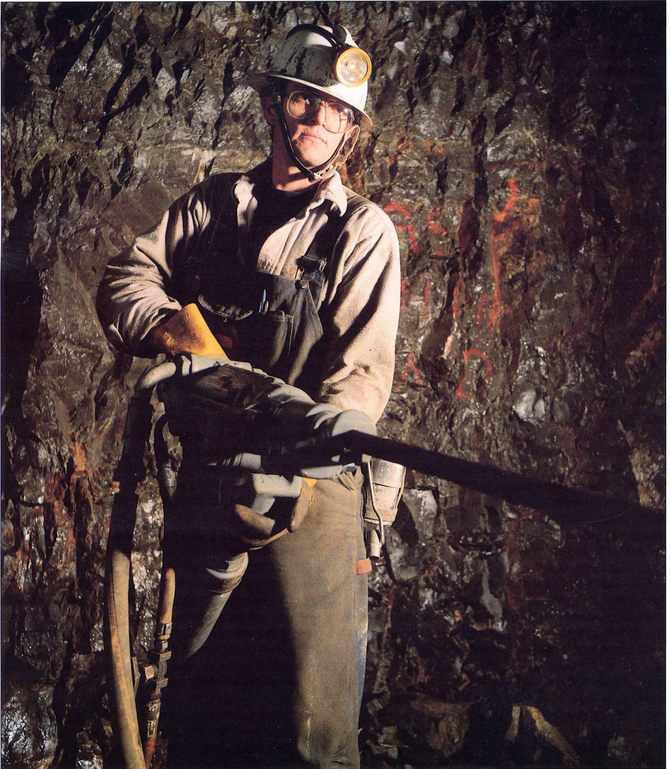
Jeff Bannister, Miner, operates a jack-leg drill in the Sullivan mine. Ore from the lower levels is being mined by conventional and mechanized methods.
