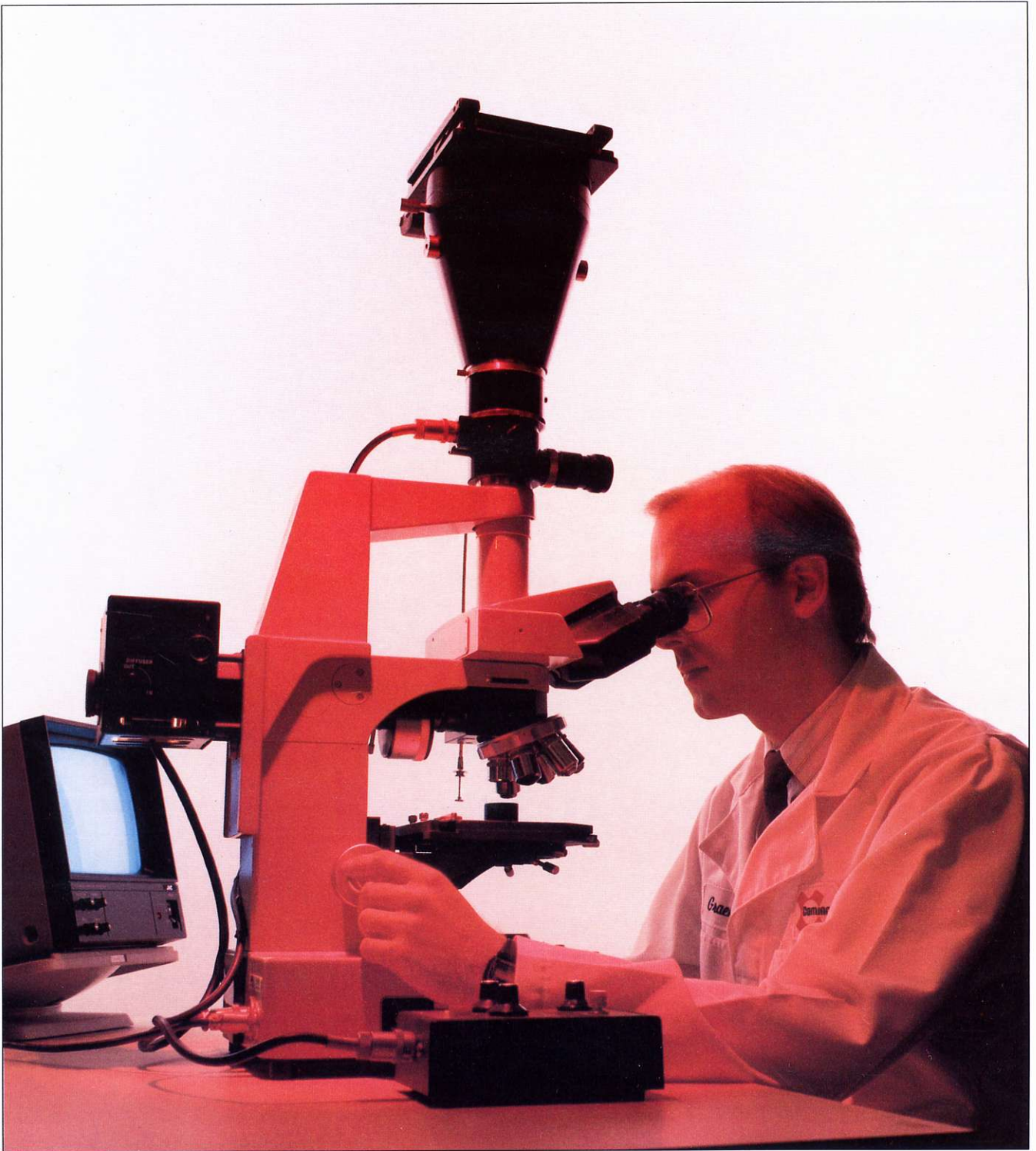
Graeme Anderson, Research Engineer, analyzes the microstructure of a zinc galvanized coating with an optical microscope at the Product Technology Centre.
