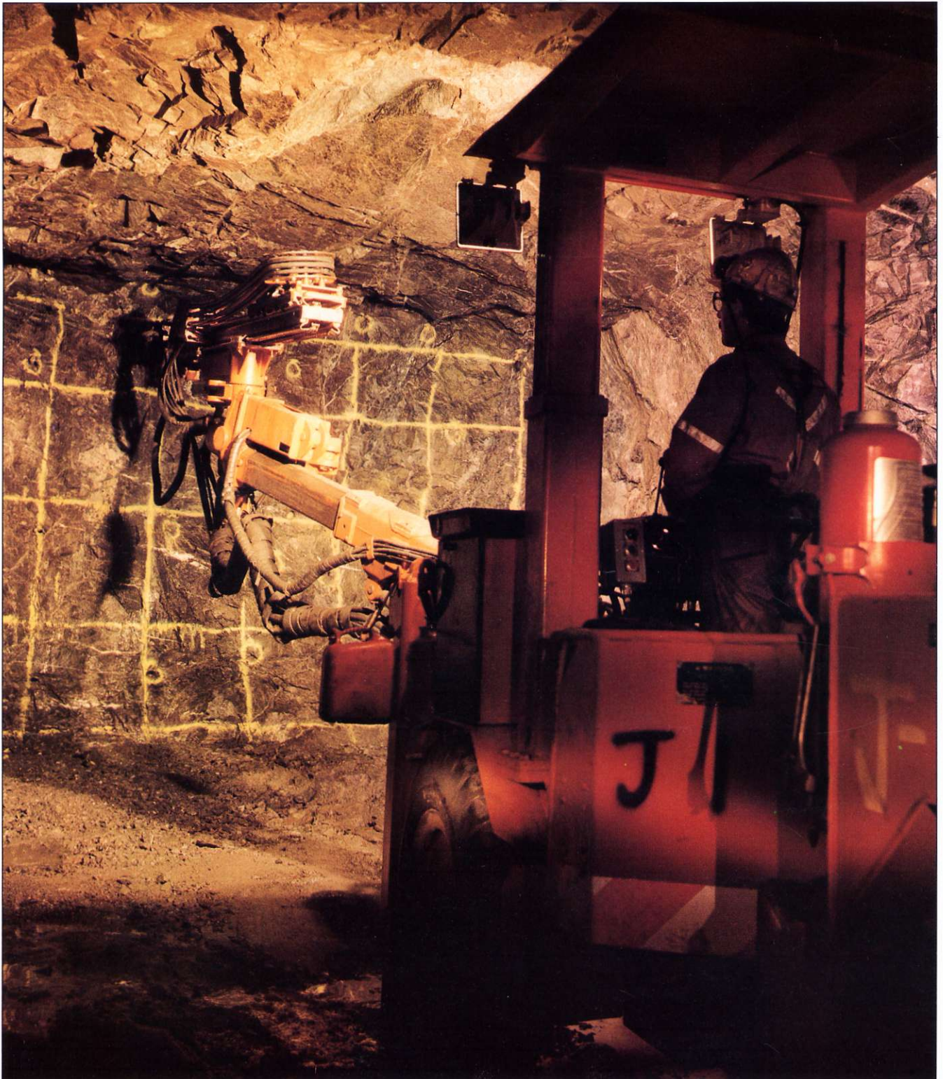
Gerry Fudge, Miner, operates a single-boom hydraulic jumbo in the 130 portal at the Snip gold mine. Production at Cominco's newest mine started January 1991.
