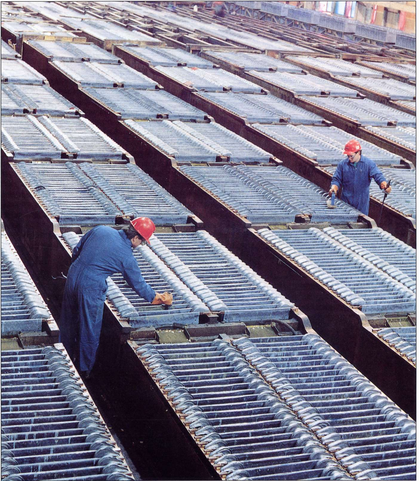
The conductivity of the electrolyte in the lead cells is tested regularly to help ensure an efficient operation in the lead refinery at Trail.
