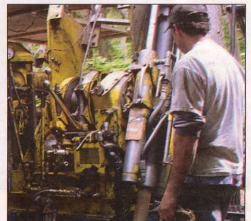
Diamond drilling at Fir property
