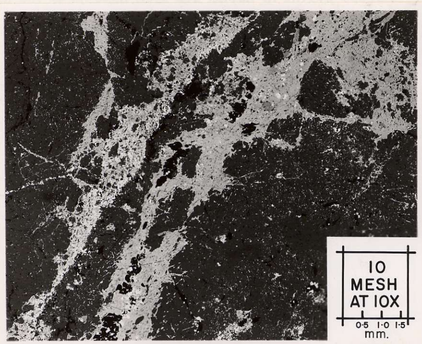
Figure 2. Photomicrograph of a polished section showing irregular masses, veins and inclusions of boulangerite (light grey) in sphalerite (dark grey). Pyrite (white) and gangue (black) are present as inclusions in both boulangerite and sphalerite.
