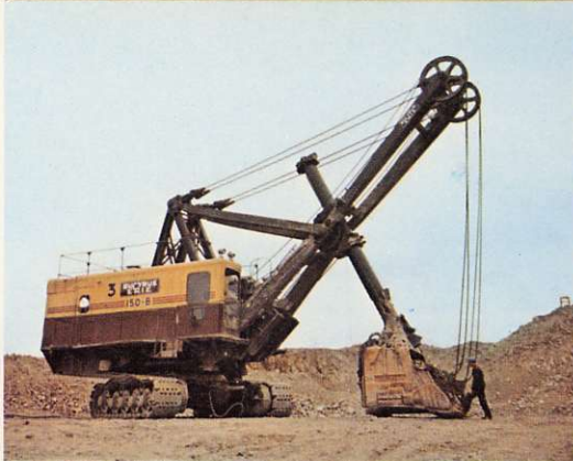
Electric shovel in the open pit. 5 cubic yards.
