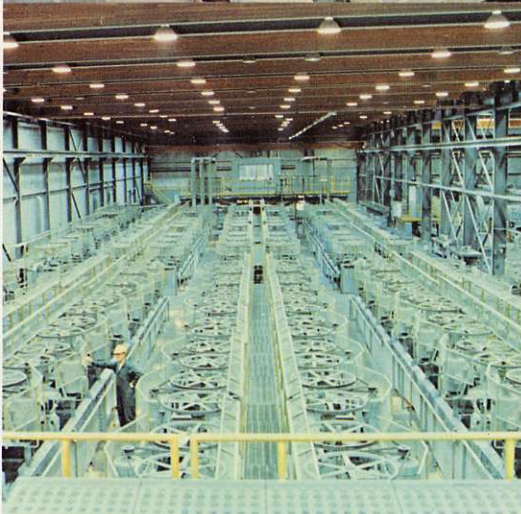
Mill concentrator flotation cells for primary separation of mineral from waste.
