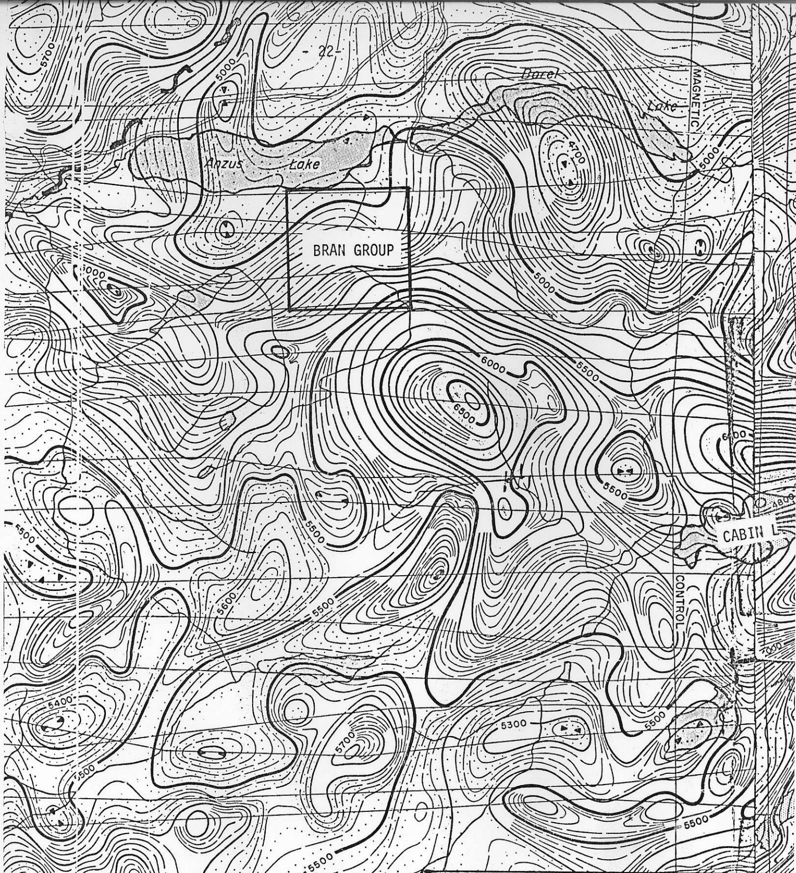
TARGET PROJECT AEROMAGNETIC MAP BOREL - ANZUS LAKE AREA 93/F Scale 1:63,360 December 1980 FIGURE 9
