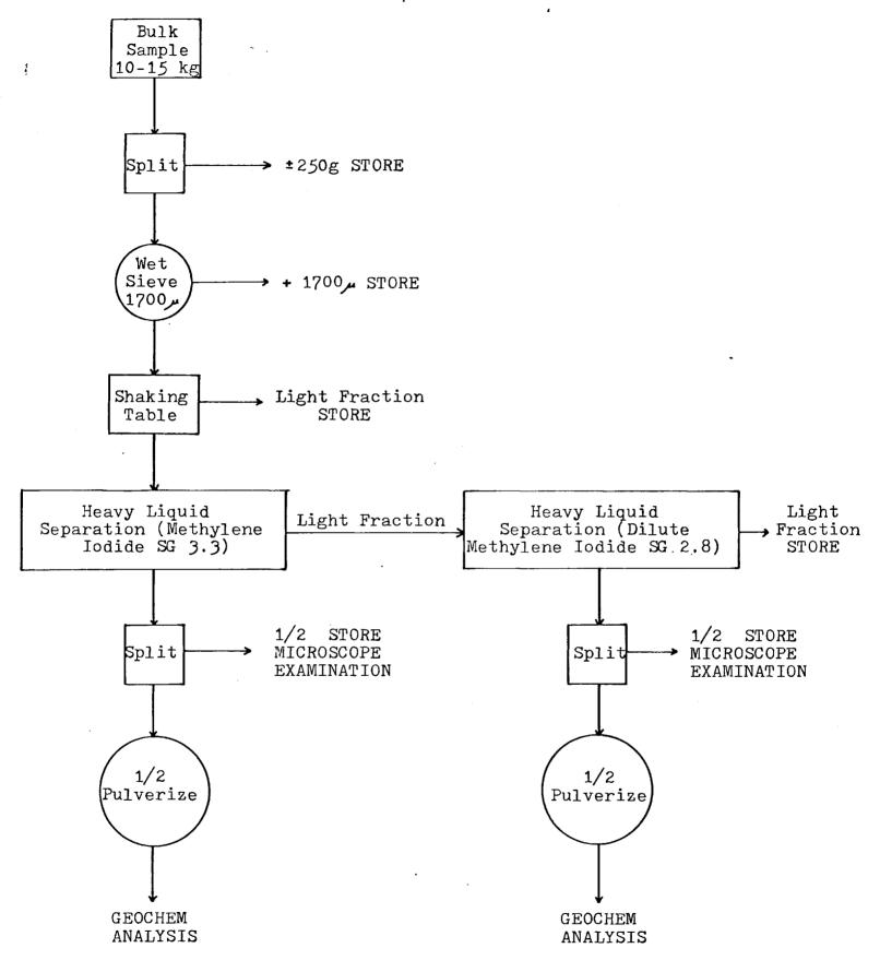
Fig. 1 - Sample processing flow sheet.
