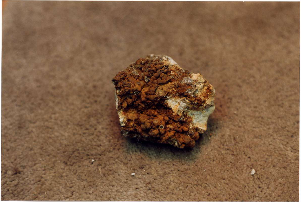
PYRITE AND BOTRYOIDAL PYRITE ON FRACTURES AND IN OPEN SPACES AROUND FRAGMENTS OF ALTERED RHYOLITE. OB #1 CLAIM
