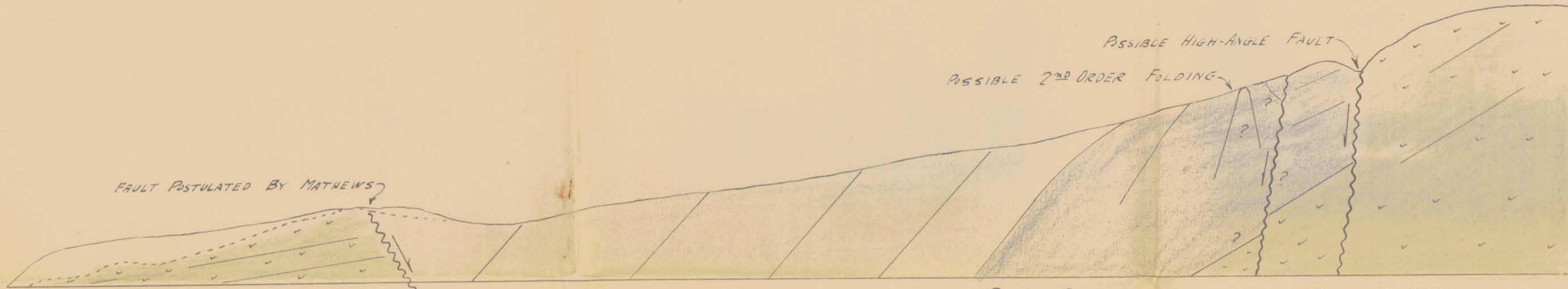
SAME SECTION AS BELOW BUT SCALE 1"=400' SHOWING POSSIBLE FAULT CONTACTS ON MARGINS OF THE LIMESTONE BELT.
