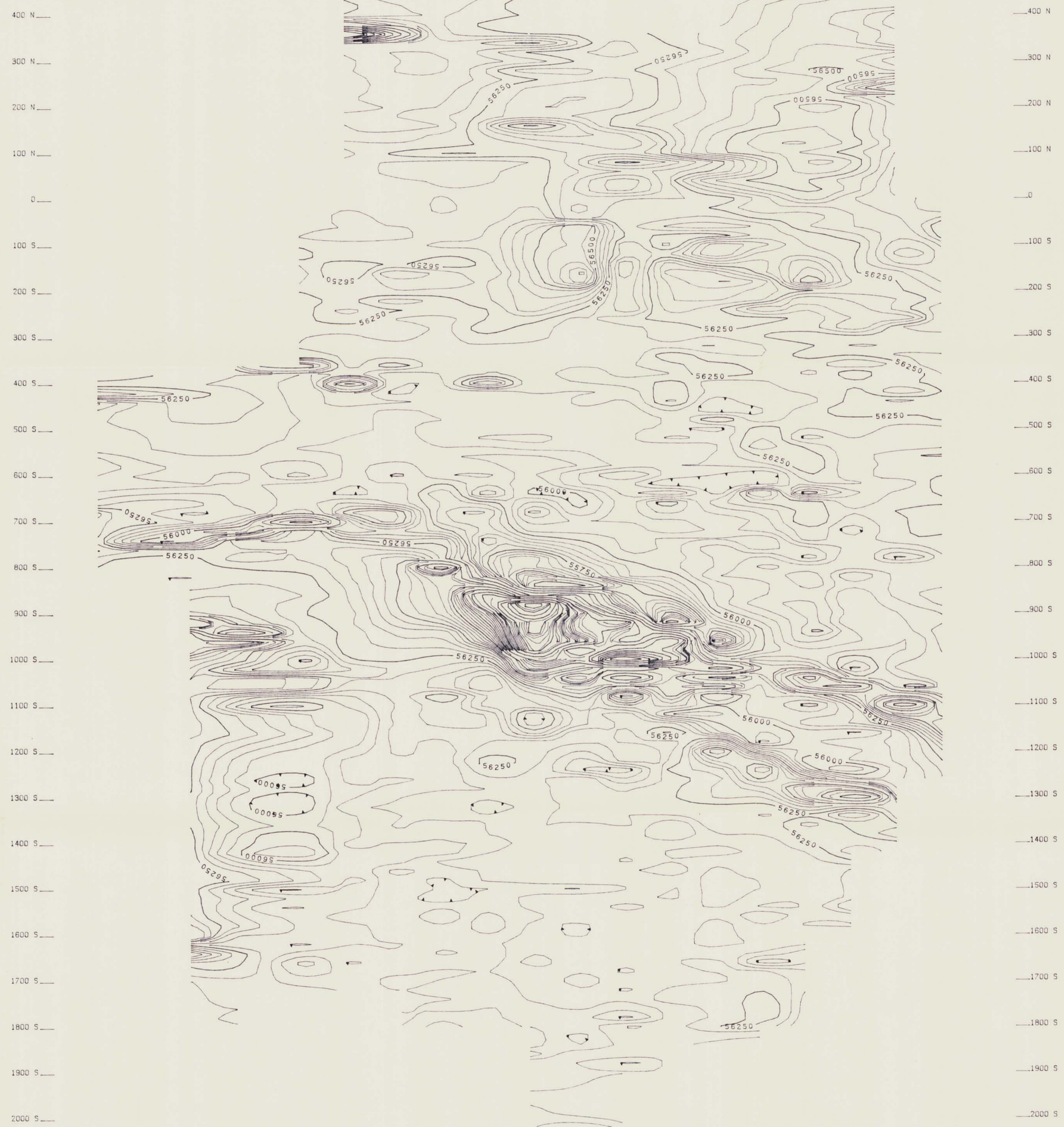
FALCONBRIDGE LTD FIG. 4 NUGGET GRID, CHEMAINUS, B.C. CONTOURED TOTAL FIELD MAGNETIC PLAN contour interval 50 nt SCALE 1:5000 DELTA GEOSCIENCE LTD
