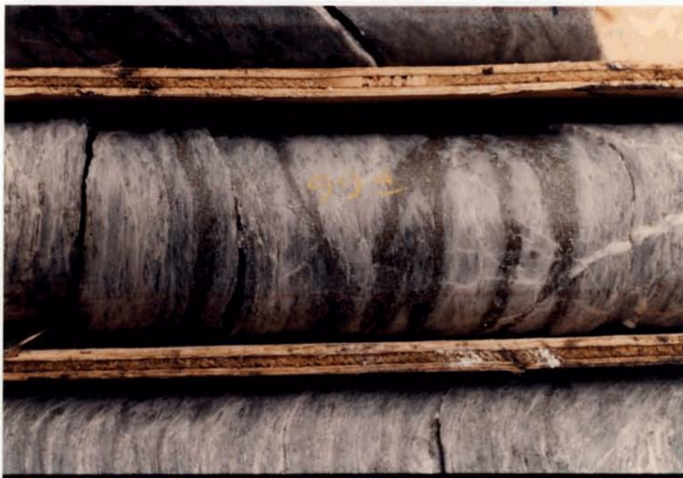
CHEM 86-18 at 99.4 m showing stringer pyrite parallel to and cross-cutting foliation at a small angle in quartz-sericite crystal tuff. Note subtle, thin alteration envelope on sulphide stringer margins.
