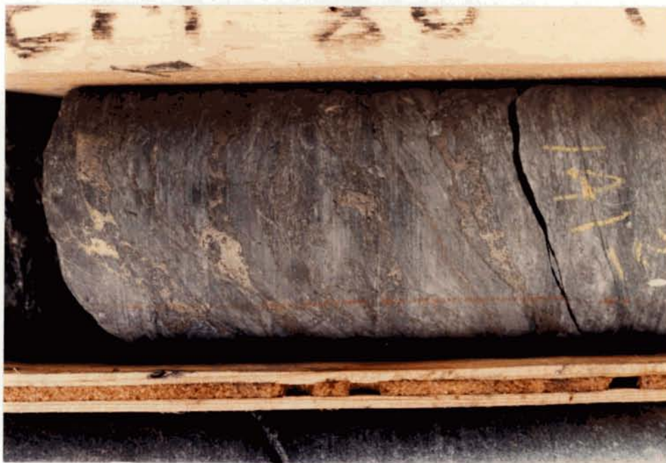
CHEM 86-18 at 141.2 m showing ragged stringers of pyrrhotite, chalcopyrite and minor, very fine sphalerite. This mineralogy is typically more common near the bottom of sulphide-bearing interval.
