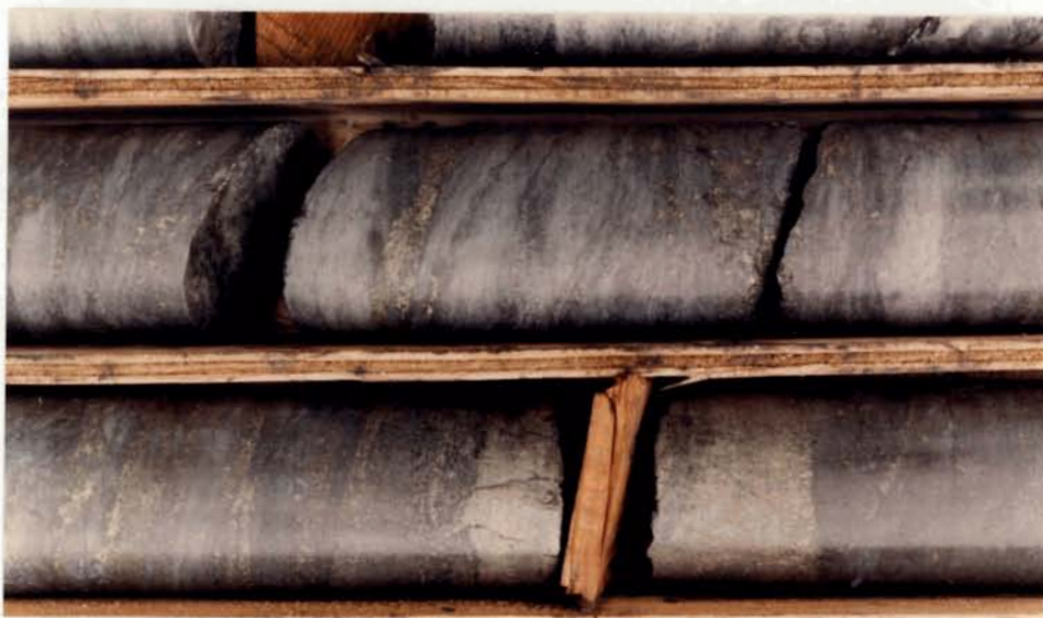
CHEM 86-18 at 136.2 m. Seams of pyrite-pyrrhotite and 4 cm wide band comprised of sub-equal pyrite and chalcopryite.
