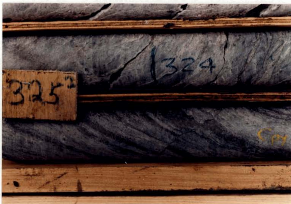
CHEM 86-14 at 325 m showing pyrite laminations parallel to foliation in quartz-sericite crystal tuff.
