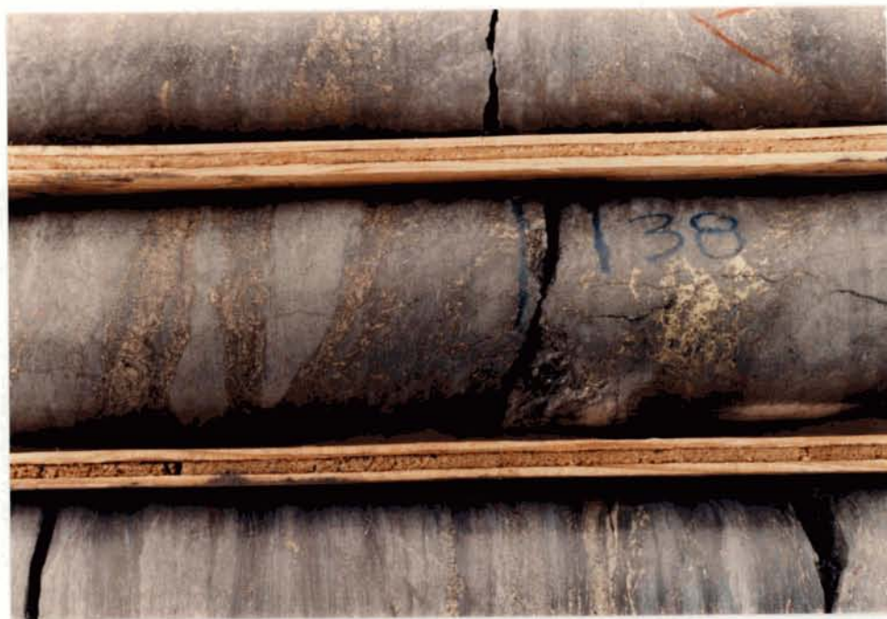
CHEM 86-18 at 138 m showing ragged pyrrhotite, pyrite and chalcopyrite stringers surrounding felsic clasts as in-situ breccia development.
