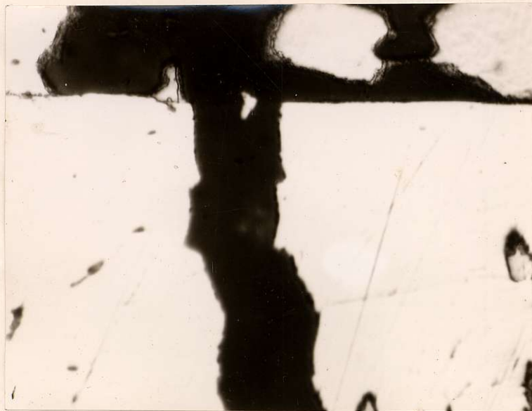
No. 1 Quartz (1) veining arsenopyrite.
