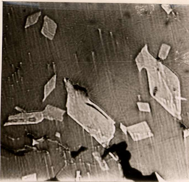
No. 3 Etched zinckenite, pseudo- morphous after arsenopyrite, enclosed in tetrahedrite X 150
