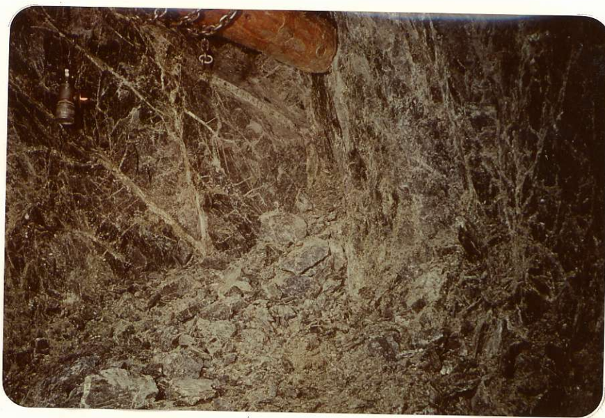
Fig. 111 Underground face showing asbestos veins in serpentine.
