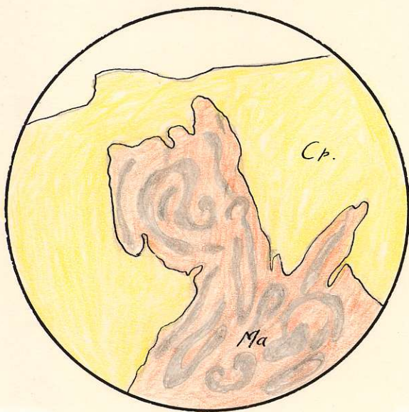
Fig. 12 Massive Marcasite (Ma) in chalcopyrite
