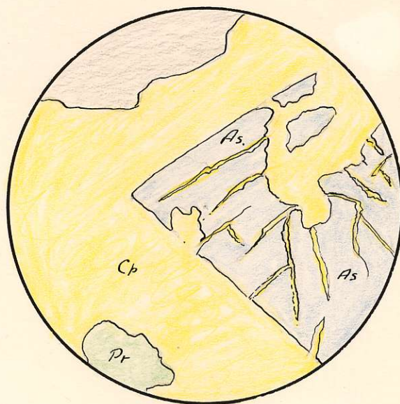
Fig. 11 Arsenopyrite (As) crystal replaced by chalcopyrite (Cp).
