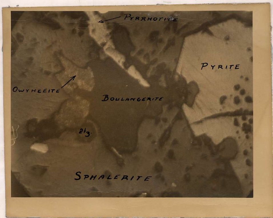
150 X Shows corrosion of euhedral Pyrite Etched 15 sec with HNO_3 , nicols partly crossed.
