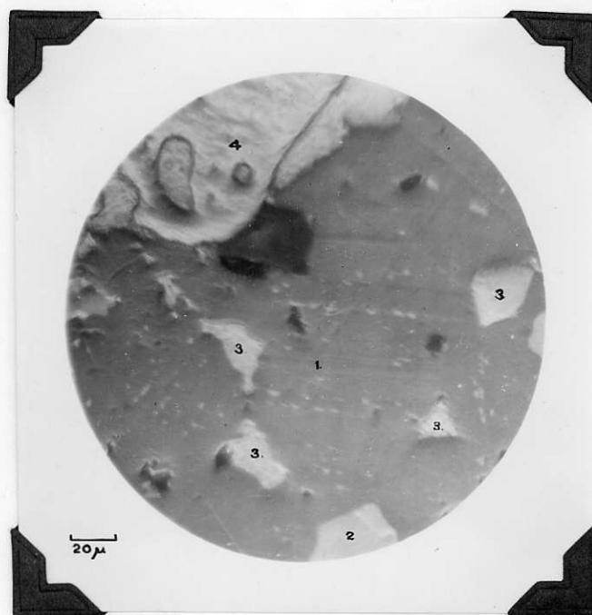
Fig 7. Chalcopyrite inclusions in sphalerite irregularly spaced along straight lines, possibly cleavage traces.
