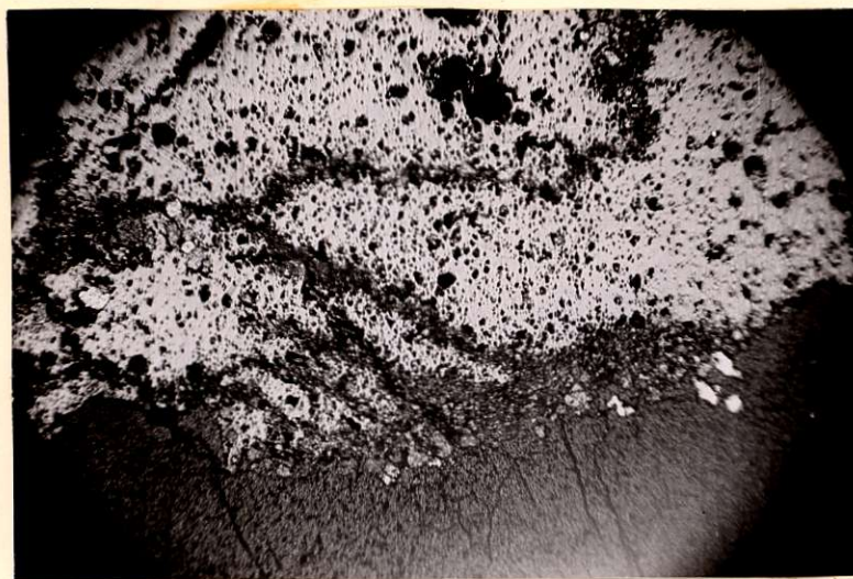
Figure 13. Ore from No. 10 Level. Pyrite (dark gray and granular) occurring as stringers cross-cutting the sphalerite (white). The pyrite has probably entered the irregular fractures in sphalerite and therefore occur as very irregular veinlets. The gray mass at the lower edge is quartz. X 50.
