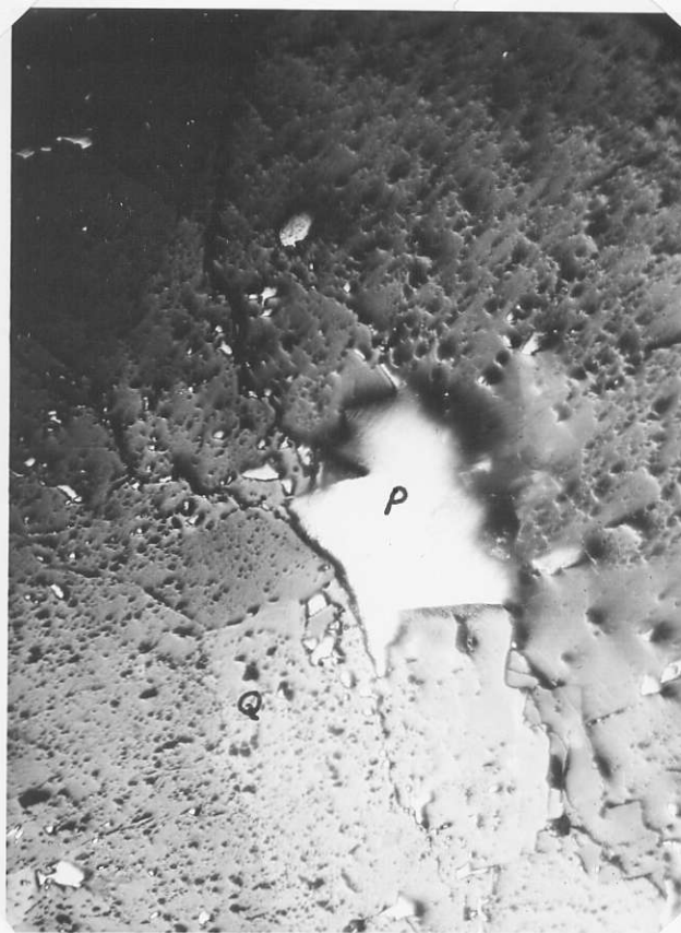
Figure 5. Photomicrograph showing pyrargyrite (P) in hematitic quartz (Q). xl65
