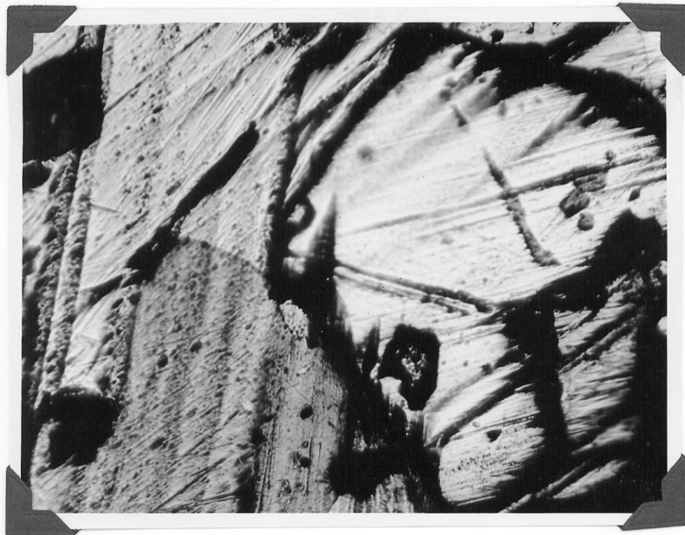
PLATE 1 Sphalerite (grey) replacing chalcopyrite lower left; Pyrite crystal above this (diam. .5mm.) also partially replaced by sphalerite as well as containing sphalerite inclusions.
