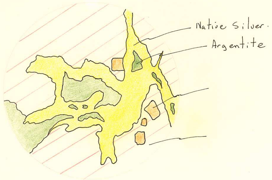
Figure 9. Native silver replacing argentite.
