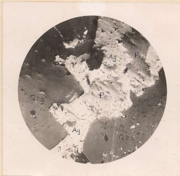
Fig. 13. Pyrrhotite (P) altering to Native Silver (Ag) in veinlet.
