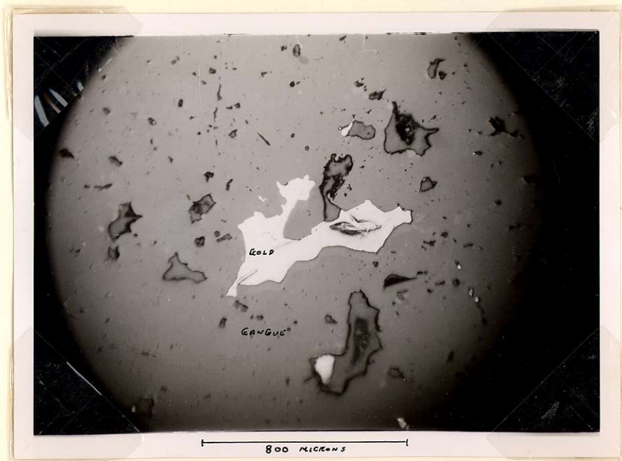
SEC. 2 LARGE "BLEB" OF GOLD WITH CHARACTERISTIC ANGULAR BOUNDARIES.
