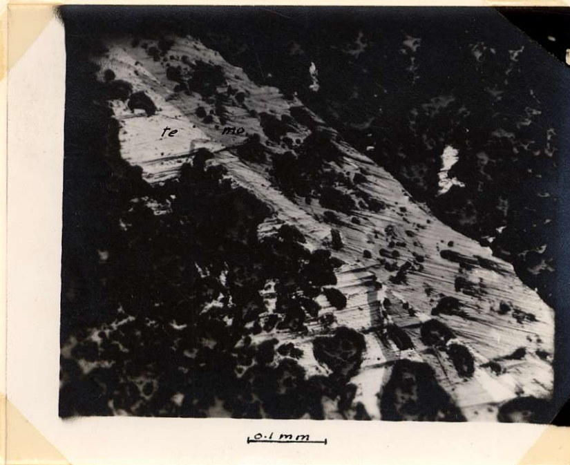
Fig. 4: Molybdenite lath with replacement of bismuth tellurides along crystal planes (Section 10)
