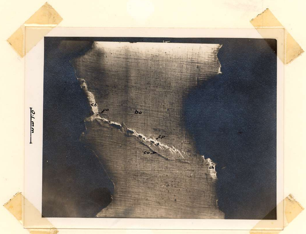
Fig. 2: Bornite (with exsolution lamellae of chalcopyrite) showing replacement by chalcocite (Section 8)
