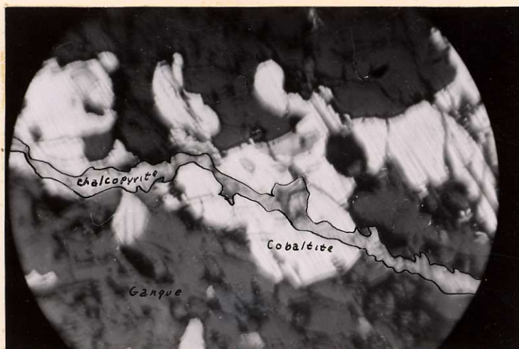
Fig.7: Chalcopyrite Cutting Cobaltite.
