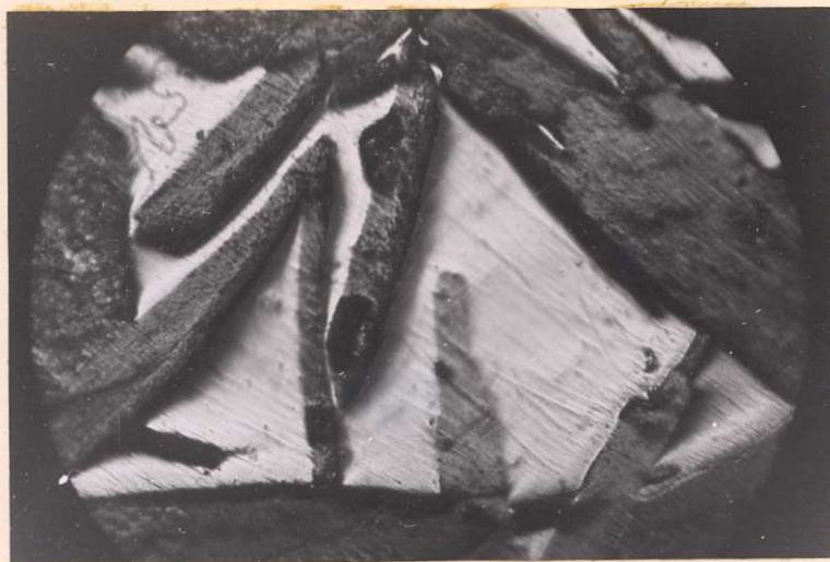
Fig.6: Molybdenite (dark grey) Replacing Chalcopyrite (white)
