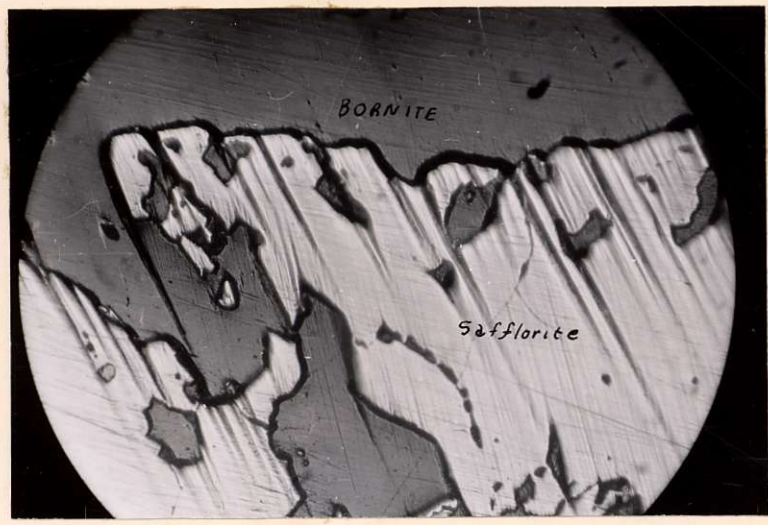
Fig.1: Bornite Replacing Safflorite
