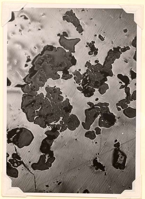
Galena replacing sphalerite. X150
