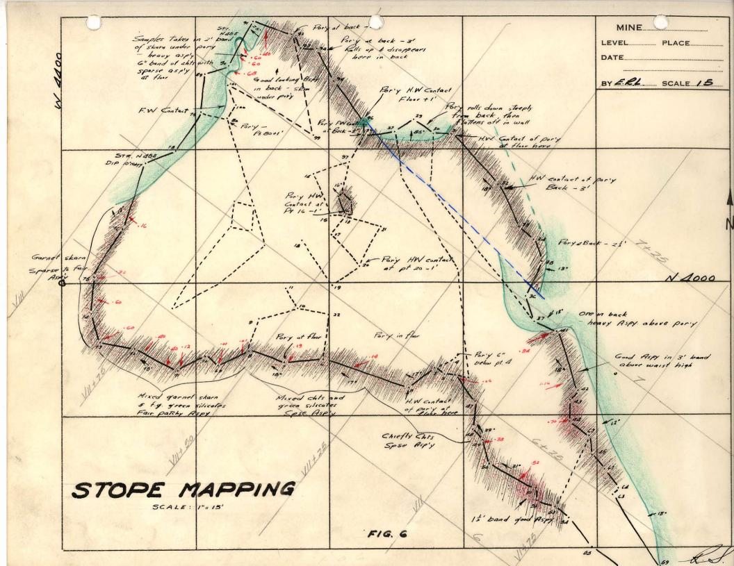
taken to irregularities in the back, walls, and floor. The slope of the tape is measured with the Brunton, and the bearing is determined by a deflection angle from a known base line. A plan and section are then drawn and the raise is mapped.
