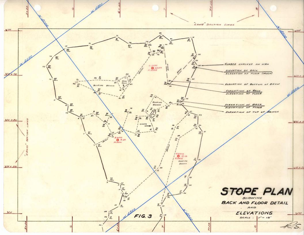
on the walls and numbered as they are surveyed; and are used as reference points in the mapping. In addition, they are used in the accurate correlation of the geological information obtained in the various parts of the mine.
