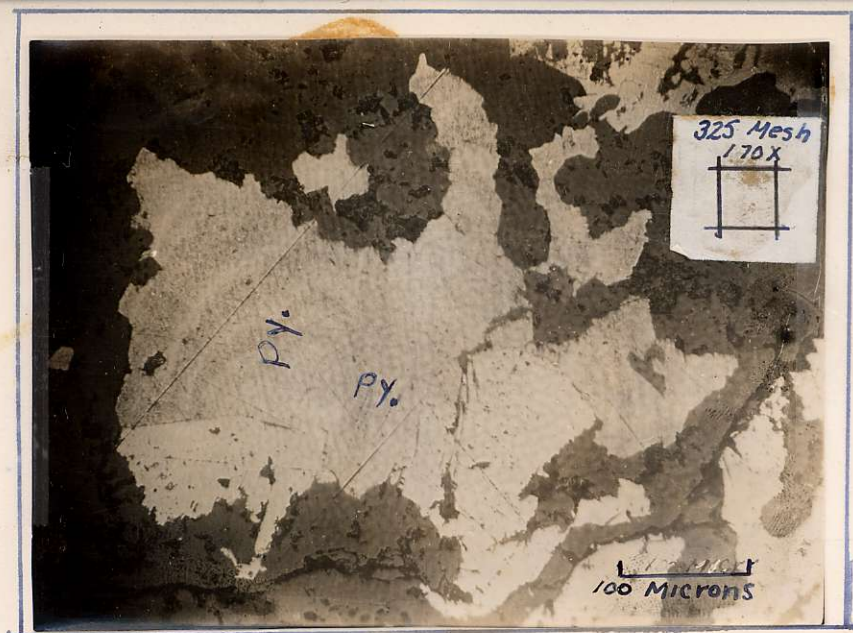
NICKEL PLATE (Photo no. 2) Section 49---Middle Red. Coloform Structure in Pyrite & Marcasite ( Magnification 170 x )
