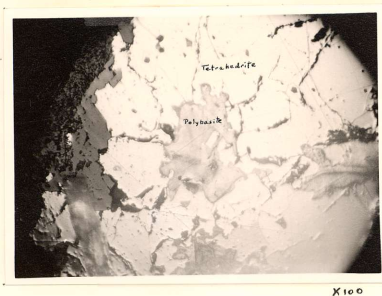
Plate 7. Polybasite (etched) in tetrahedrite
