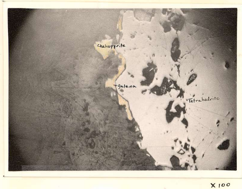
Plate 6. Galena, showing cubic cleavage as rim at edge of Tetrahedrite grain.
