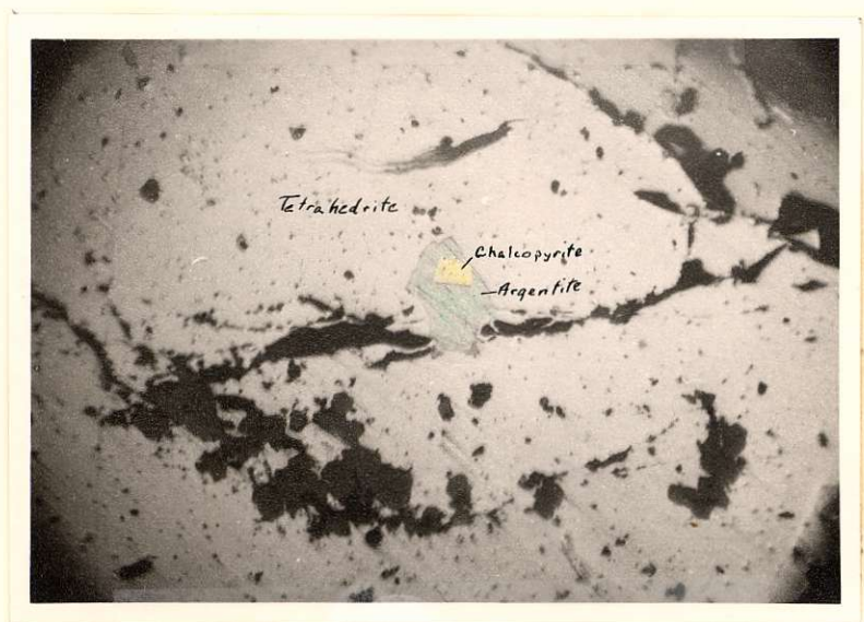
Plate 10. Exsolution of Chalcopyrite from Argentite, from tetrahedrite
