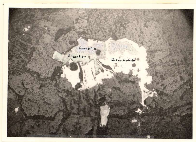
Plate 5. Covellite replacing Argentite, an exsolution product of Tetrahedrite
