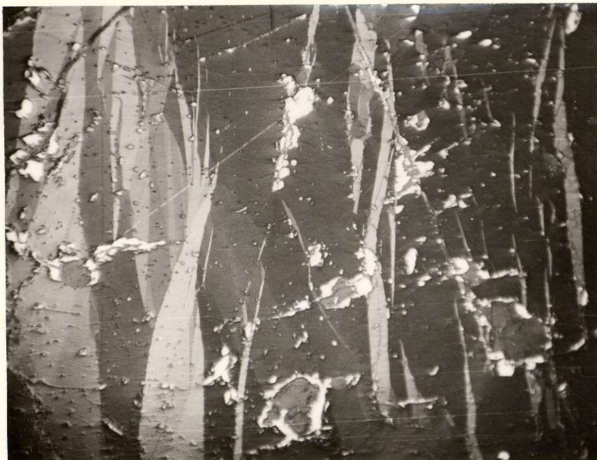
Plate 5. Stress twinning in pyrrhotite. (crossed nicols) X80
