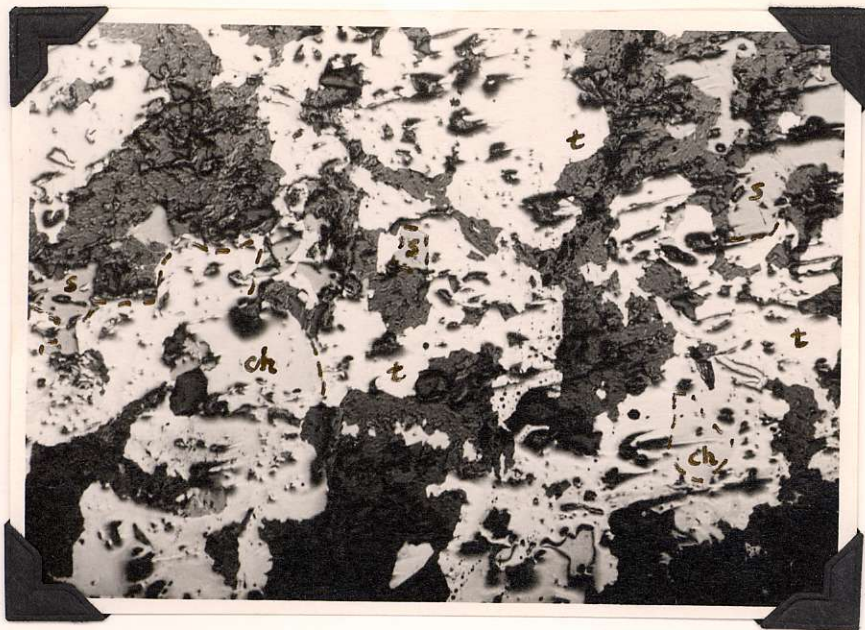
Section No 2. Intergrowth of Sphalerite, chalcopyrite and tetrahedrite
