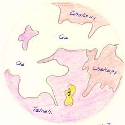
Fig. 2 # 7 vein Galena replacing tetrahedrite. Chalcopy. replacing tetrahedrite & galena.
