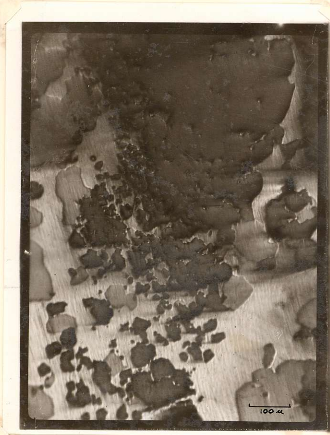
Figure 1. Replacement Texture Showing Galena Replacing Sphalerite
