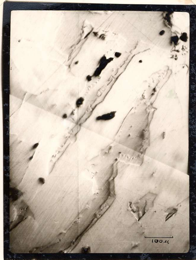
Figure 3. Tetrahedrite Grains Surrounded by Bournonite in a Matrix of Meneghinite
